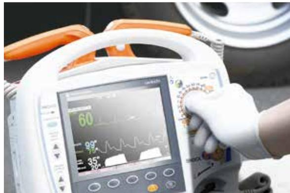
Conventional display: 450 cd/m<sup>2</sup>, TEC-5600 display: 1000 cd/m<sup>2</sup>
